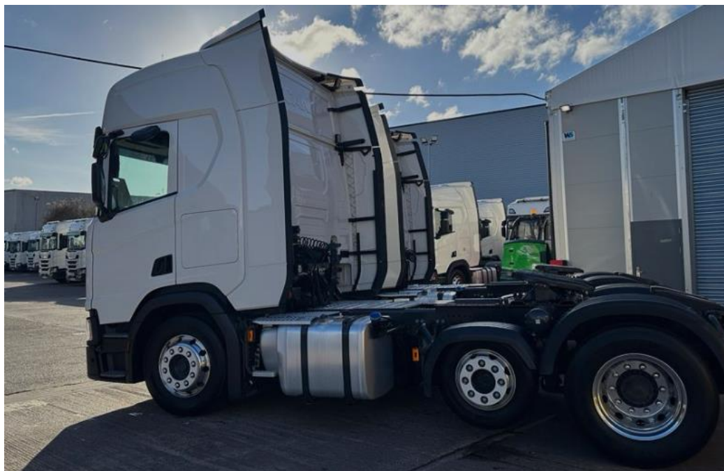
Figure 8: Example of a UK spec 6x2 “Mid Lift” tractor unit
