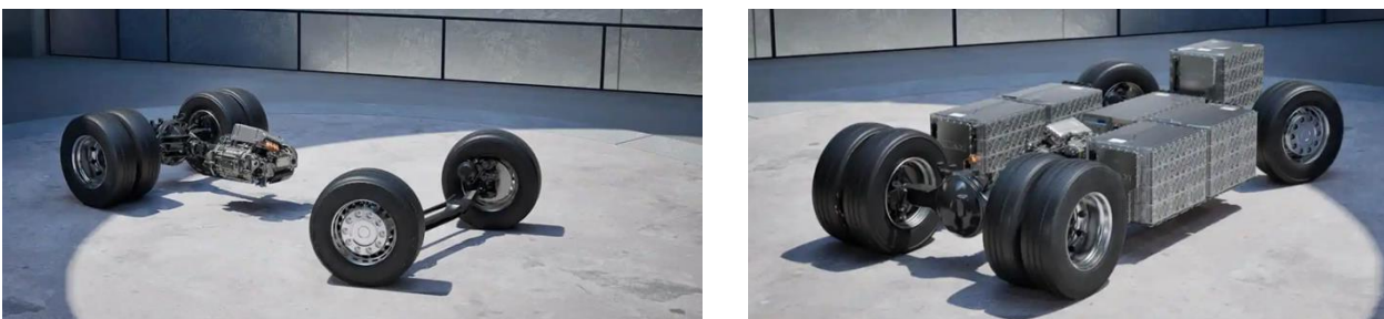
Figure 2: Illustration of electric motor and gearbox position (left) and with battery packs and inverter (right).
