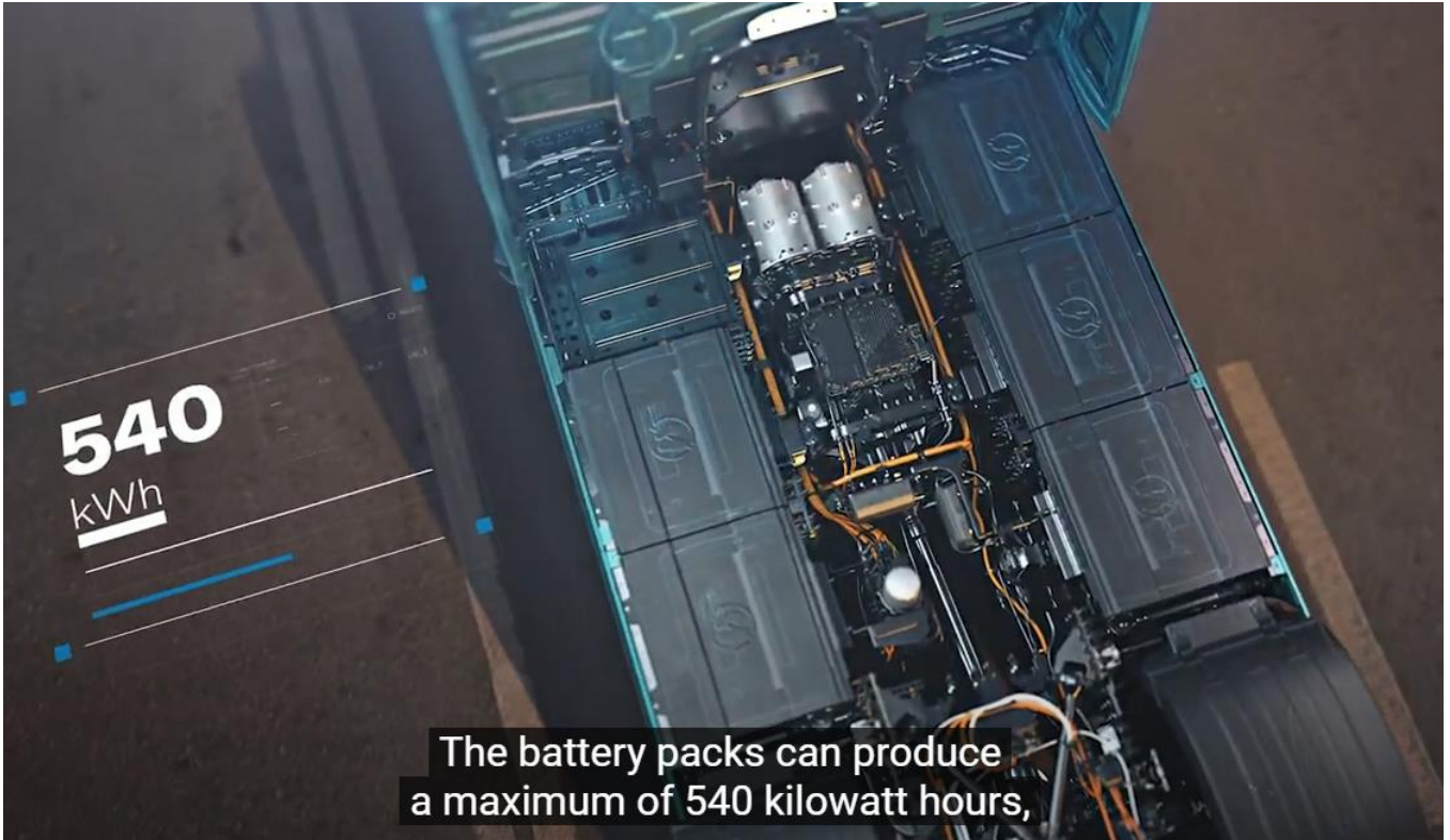
Figure 1: Layout of electric motors, gearbox and battery packs in Volvo’s first FH Electric units. Source: Volvo YouTube video 4
