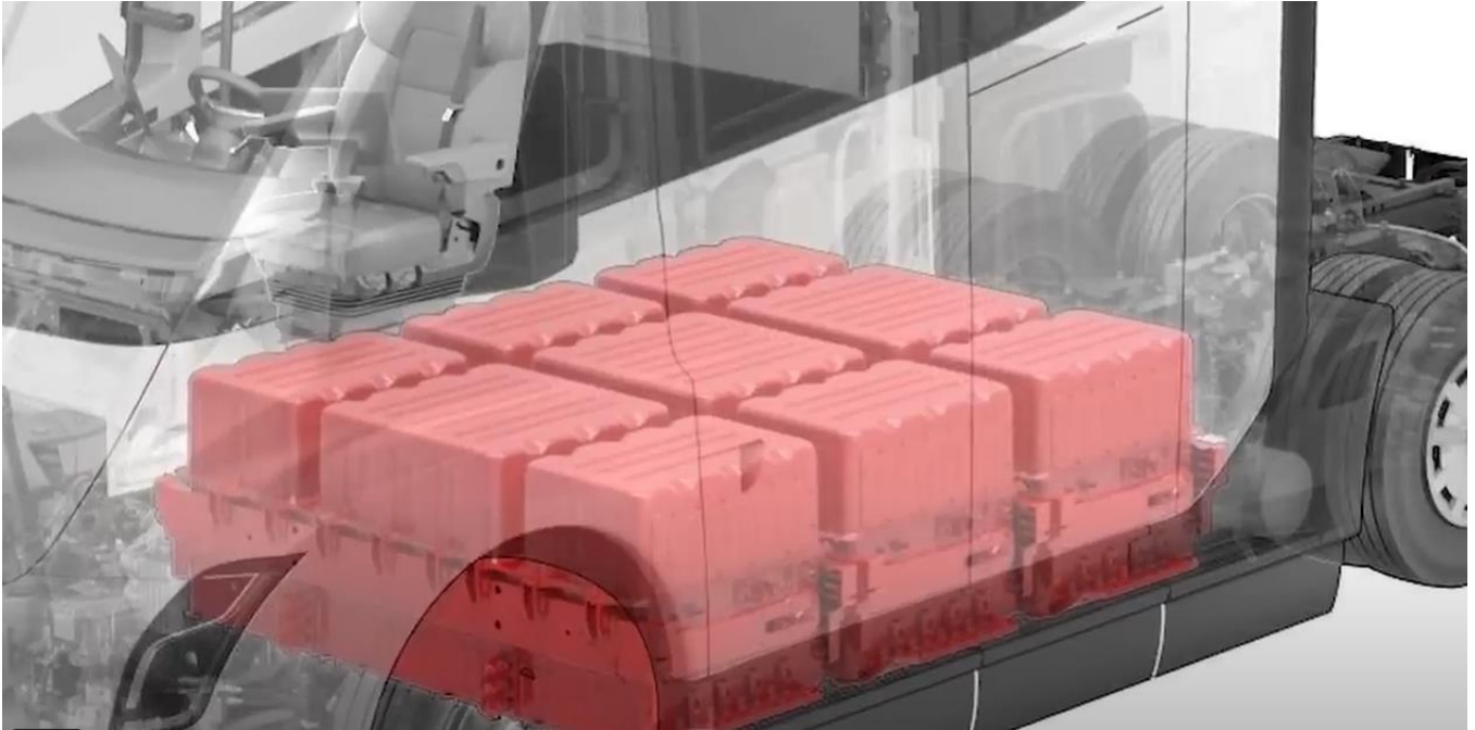
Figure 10: Illustration of the location of the Tesla semi-battery packs. Source: Unverified internet
